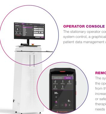
The stationary operator console offers general system control, a graphical user interface for patient data management and a safety stop.
